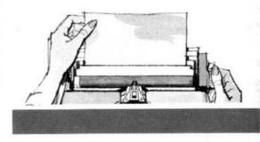
Freeing the paper with the Paper Release Lever, move it horizontally until the character is bisected by the white line on the Line Indicator. Return the Variable Line Space Button and the Paper Release Lever to normal position and typing will be in perfect alignment.
