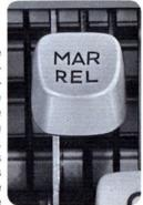
typing. Should you strike two keys at the same time, the type bars may lock at the printing point. To free the type bars, simply depress the margin release key.
