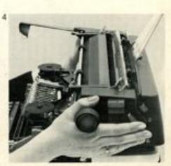
Remove the red screws on either side of the carriage guide rails. (Fig. 7). Move the carriage to the right and remove the four locking pieces.
