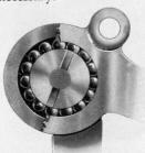
Note the fifteen hardened steel balls in this type-bar bearing, which is partially cut away to show the nice construction and the perfectly fitting, adjustable cone. These balls are made in our own plant, with such precision that there is not one ten-thousandth of an inch difference between them.
