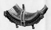
When you shift for capitals on the L C Smith, this segment or "type-bar basket" is all that moves, regardless of width of carriage. The carriage remains solidly on the frame. No vibration, and the minimum of effort.
