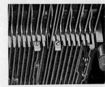
The two adjustable stops shown in this underneath view of the machine prevent the period and comma from perforating the paper.
